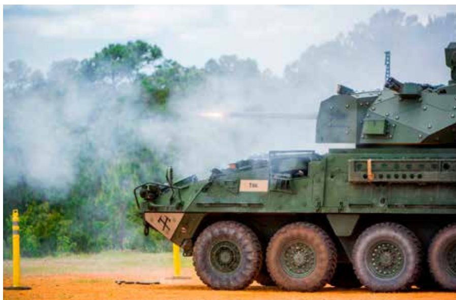
Medium Caliber Weapons System demonstration by the Army Armament Research, Development and Engineering Center aboard the MCoE. Nearly identical to the 30mm cannon on the future amphibious combat vehicle, the Medium Caliber Weapons System is designed to enhance the accuracy and lethality of the M1126 Stryker Combat Vehicle. (Photo by Patrick A. Albright.)
