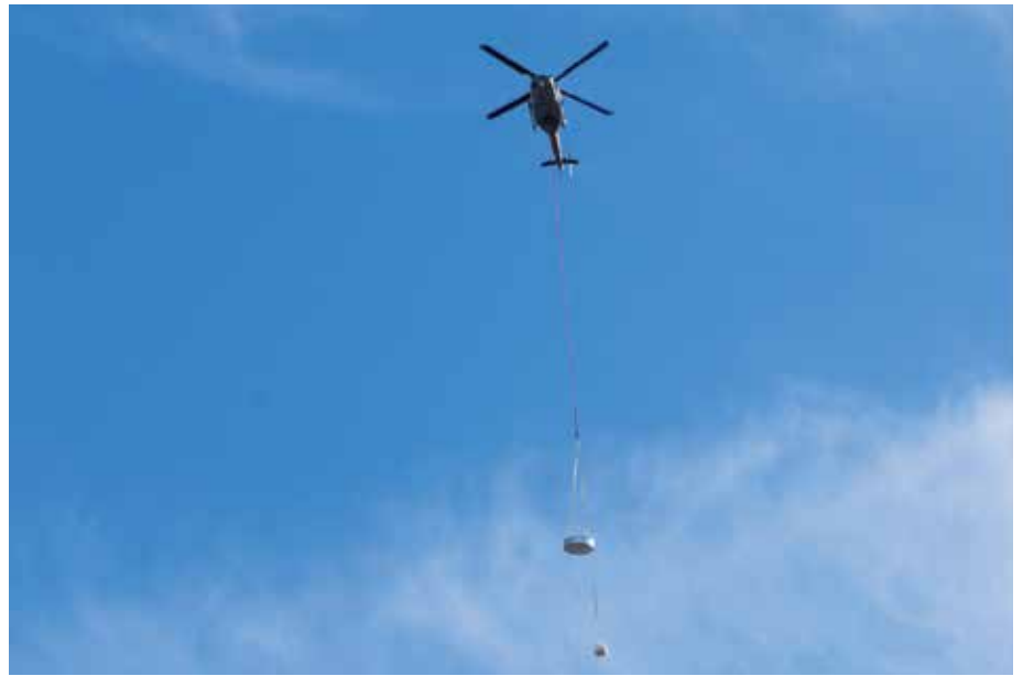
UH utilizing the longlines with specialized weight. (Photo by Mr. Brian Schwab.)
