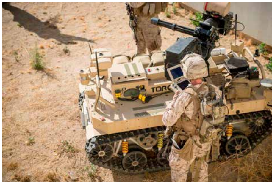
Marines with a weaponized multi-utility tactical transport (MUTT) vehicle during experimentation at Camp Pendleton. (Photo by LCpl Julien Rodarte.)
