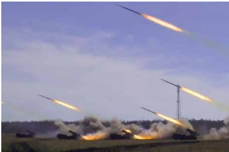
BM-27 Uragan 220mm multiple launch rocket systems firing during a Russian military exercise. Timelines associated with coordinating fires using such longer range systems are still very responsive. (Image from RT.)
