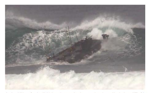
An Amphibious Combat Vehicle undergoes developmental testing at Vandenberg AFB, CA. (Photo by Douglas Kenner.)
