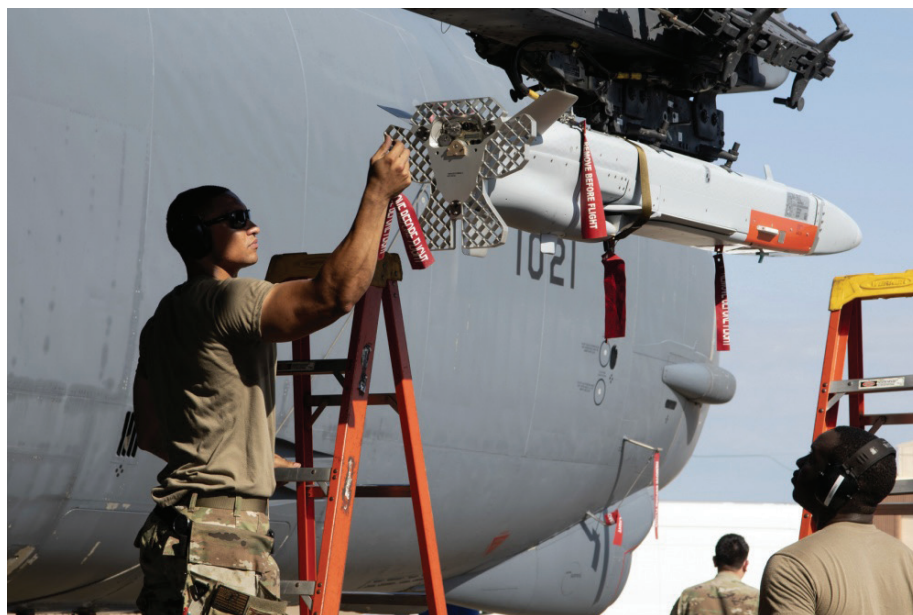
Use of decoys like the Miniature Air-Launched Decoy (MALD) ADM 160X is nothing new. (Photo by Airman 1st Class Celeste Zuniga.)
