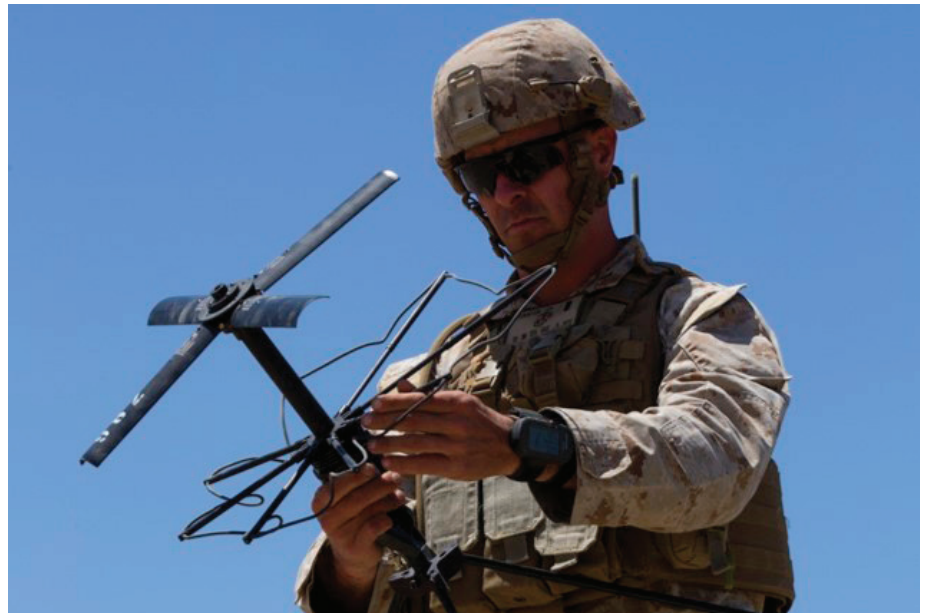
1stLt Adam Fountain sets up a SATCOM antenna to communicate with his sniper teams at ITX. (Photo by author.)
