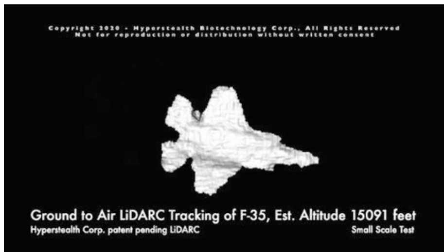
Figure 3. Ground-to-Air LADAR of F-35 at 15000 feet. Used with permission. (Figure provided by authors.)
