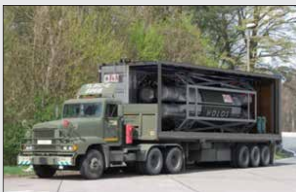
Figure 4. Holos micro reactor onboard a flatbed. The Holos microreactor can be scaled from a minimum of three MWe to a maximum of thirteen MWe for Holos Quad generators and comprised within a single transport container. The Air Force intends to field a similar prototype micro nuclear reactor at Eielson AFB, AK, by 2027 to allow that remote site to reduce reliance on coal. 17 (Information available at ImageForbes.com and holosgen.com .) (Figure provided by author.)
