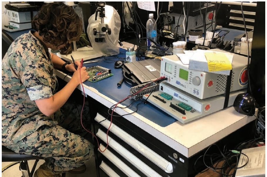
Cpl Garcia, with 2d Maintenance Battalion, Electronics Maintenance Company, inspects electronic components with the Circuit Card Assembly Test Station aboard Camp Lejeune, NC. Marines have averted $15.2 million in replacement part costs over the past five years by organically repairing circuit cards. (Marine Corps photo by Matt Gonzalez.)
