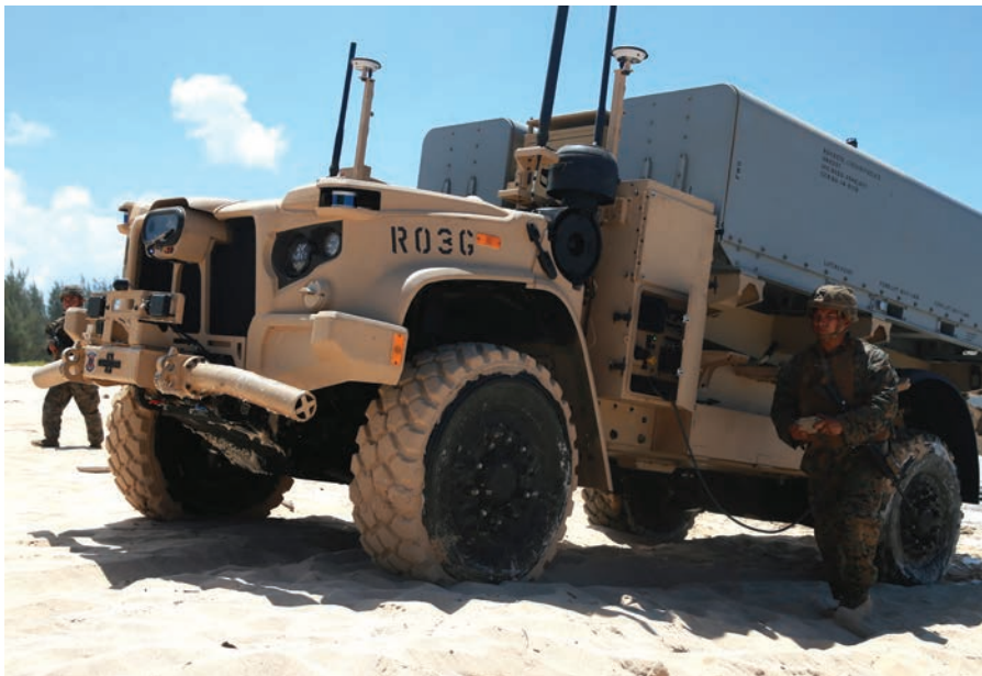
An artillery Marine maneuvers a Navy Marine Expeditionary Ship Interdiction System (NME-SIS) launcher which can provide Marine Stand-in Forces a proven capability to strike a naval target from more than 100 nautical miles. (Photo by Cpl Luke Cohen.)
