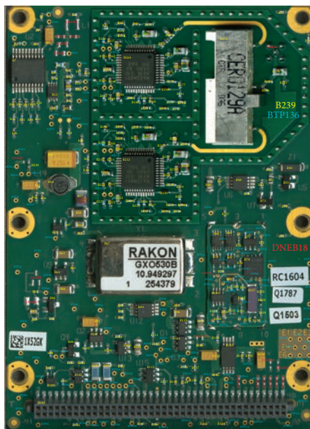
A close-up view of a multi-layer circuit card with labeled surface-mounted components. This type of information is a critical component of a technical data package. (Photo provided by Phillip Comer.)
