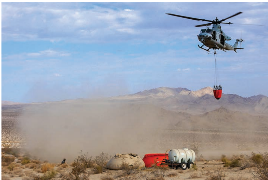
UH with standard configuration drawing water from the pumpkin. (Photo by Mr. Brian Schwab.)
