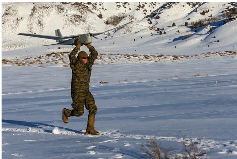
Force Design 2030 optimizes the Marine Corps for reconnaissance-strike tactics. A Marine launches an RQ-20 Puma sUAS during Mountain Warfare Training. (Photo by Cpl Eric Tso.)
