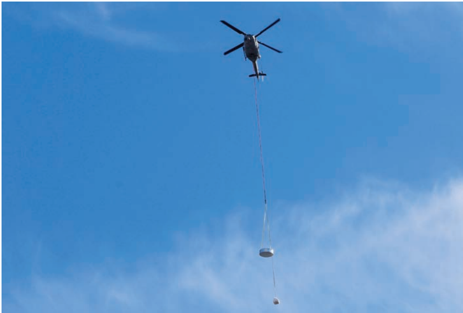
UH utilizing the long-line with specialized weight. (Photo by Mr. Brian Schwab.)
