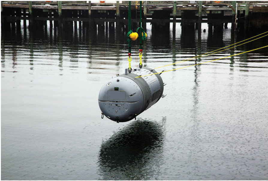
An autonomous submarine being tested, the large displacement unmanned undersea vehicle, "Snakehead," provides a variety of capabilities including sensors in support of intelligence preparation of the operational environment. (Photo by Richard Allen.)
