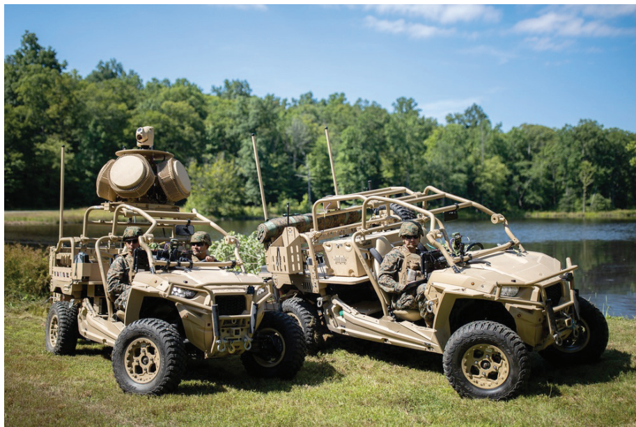
The Light-Marine Air Defense Integrated System (L-MADIS) provides both kinetic and non-kinetic defeat capabilities to destroy or negate aerial threats. (Photo by Tia Dufour.)
