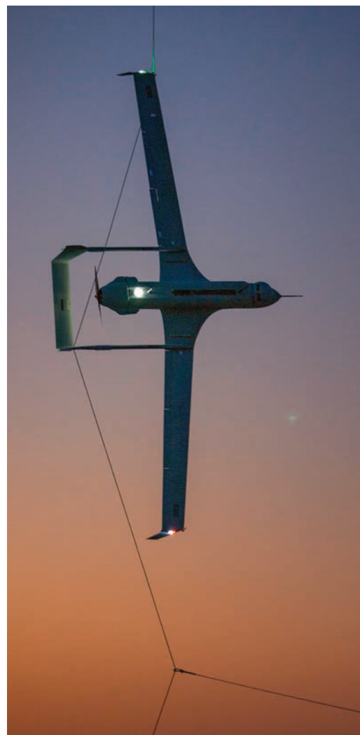
An RQ-21A Blackjack is caught by a cord to safely land at Nackeroo Airfield, Northern Territory, Australia, Aug. 12. The UAS can provide surveillance and reconnaissance to Marines on the ground and was a vital asset during Exercise Looby. (Photo by Cpl Lydia Gordon, USMC)
