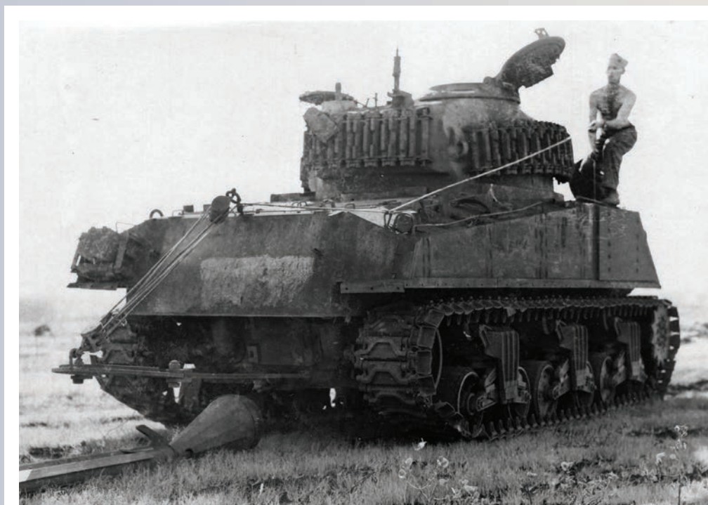
Marines of Company A, 4th Engineer Battalion attach an explosive “snake” to an M4 medium tank. The snake appears to be an adaptation of a Canadian mine-clearing line charge of the same name—essentially an oversized Bangalore torpedo. The Marine version could be pushed or pulled into position by a tank. This photo was taken at Camp Maui in 1945; note the tank still sports additional armor from the fighting on Iwo Jima. (Photo by PFC James B. Cochran, USMC)
