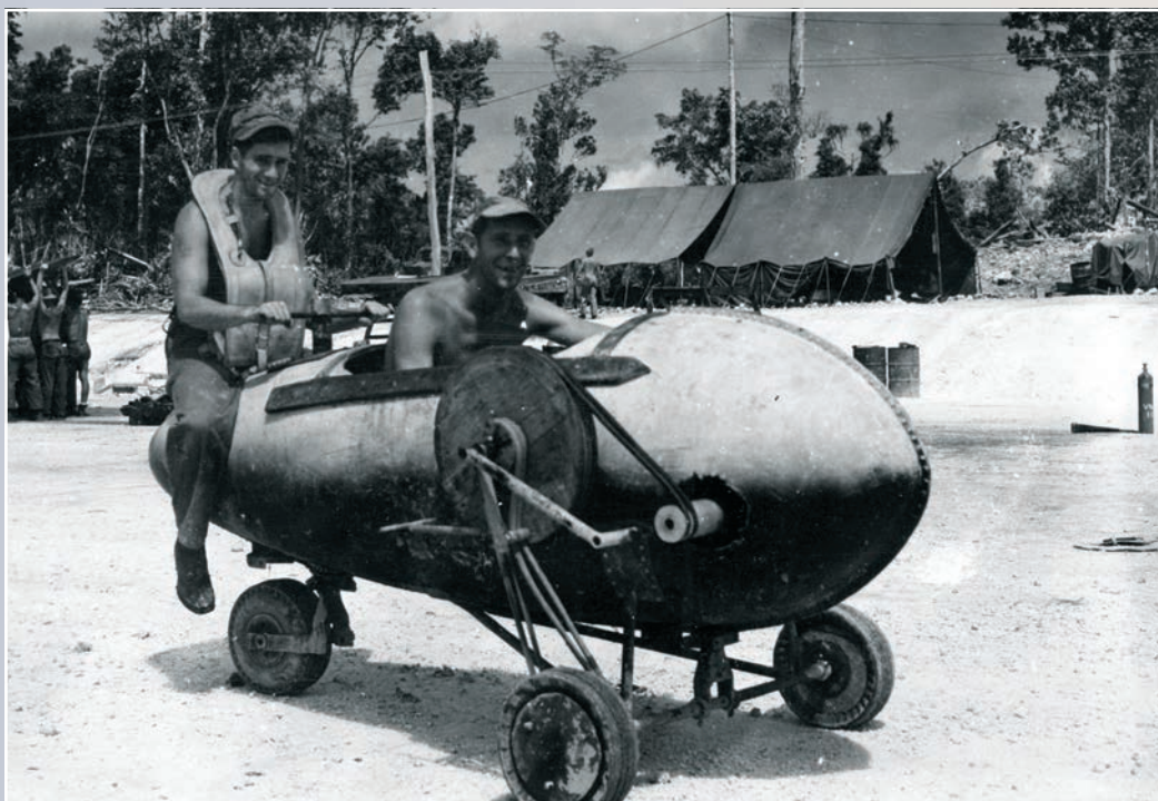
The “Galloping Gas Tank” was built by Sgt Andrew J. Moynihan, left, and Sgt Robert H. Oatley, right, VMF-115 crew chiefs at Emirau in July 1944. The sergeants owned a horse and cart on Guadalcanal, but had to leave their conveyance behind when the squadron moved. The inventive pair equipped a discarded fuel tank with a one cylinder motor and could cruise along the flight line at 20 miles per hour. (Photo by TSgt Gordon G. Greitzer, USMC)
