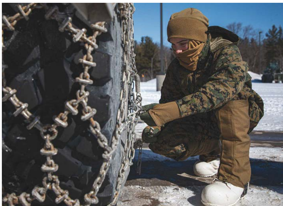
LCpl Gabby Seman tightens snow chains during a snow chains assembly course, part of a cold weather exercise at Fort Drum, N.Y., March 4. Following Basic Cold Weather Leaders Training at MCMWTC Bridgeport, Calif., the Marines of CLB-8 shared their knowledge by facilitating cold weather survival and motor transport courses at Fort Drum for Marines with 2nd MLG.
