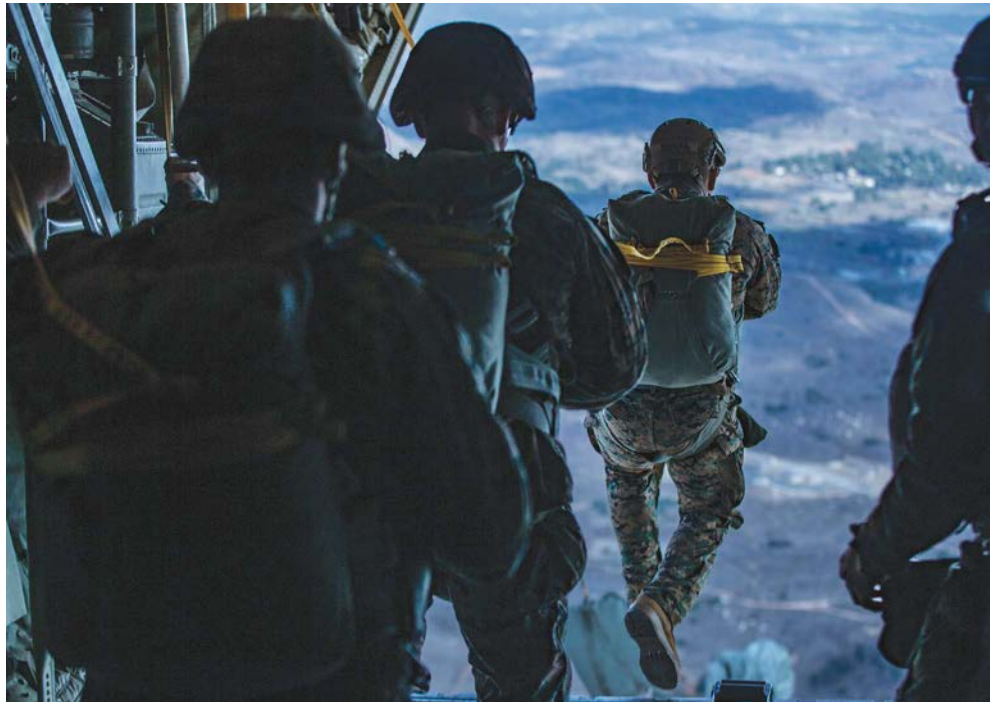
Marines prepare to static line jump from a KC-130J over Drop Zone Basilone at MCB Camp Pendleton, Calif., Dec. 10, 2020. During a static line jump, Marines' parachutes are attached to the aircraft with a cord, which deploys the canopy during the jump and enables a safe landing. (Photo by LCpl Drake Nickels, USMC)
