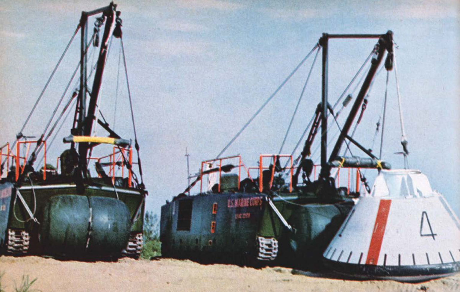
Above: Amtrac retrievers and a replica of the spacecraft before a practice run. Marines arrived at Cape Kennedy about two weeks prior to each mission's launch to ensure they were prepared for any possible problems.
