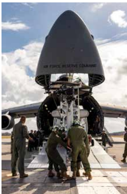
Marines and airmen load a UH-1Y Venom helicopter onto a C-5 Super Galaxy aircraft during a static load exercise at Naval Air Station Joint Reserve Base New Orleans, Belle Chasse, LA. Marine Light Attack Helicopter Squadron (HMLA) 773, 4th Marine Aircraft Wing, Marine Forces Reserve, trained alongside 26th Aerial Port Squadron, 68th Airlift Squadron, to mentor and develop the next generation of logisticians, while fostering cross-Service knowledge and collaboration between Air Force and Marine Corps teams. (Photo by Sgt Emely Gonzalez.)
