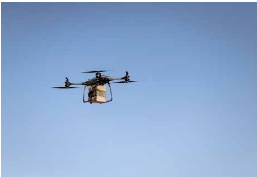
A Marine Tactical Resupply Unmanned Air System flies with three water jugs for the rapid resupply of small units in hard-to-reach locations. (Photo by Cpl Damian Oso.)
