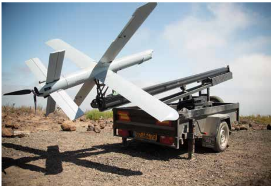
A U.S. Marine Corps Hero-400 loitering munition drone a loitering munition that the United States Marine Corps is beginning to incorporate into specific mission sets. (Photo by LCpl Daniel Childs.)
