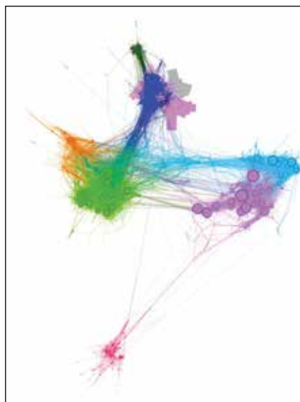
Figure 5. Network of 5,793 vessels suspected of IUUF's 26,051 at-sea encounters. Nodes are sized by being central among other highly central vessels, indicating influence (PageRank Centrality), and color is based on algorithmically defined groups (Louvain Community Detection). 20 (USMA CDT Angelina Pfister in support of TRADOC G-2, data is publicly available from Global Fishing Watch https://globalfishingwatch.org/datasets-and-code .)
