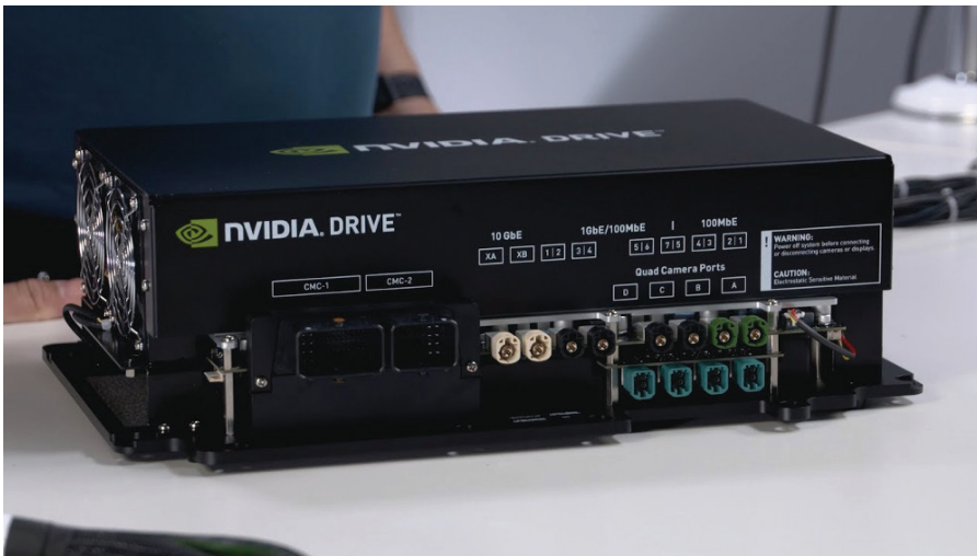
Figure 2. NVIDIA Drive is a 320 trillion operations-per-second supercomputer designed for Level 4 and Level 5 autonomous systems, including robotaxis. (Photo provided by author.)
