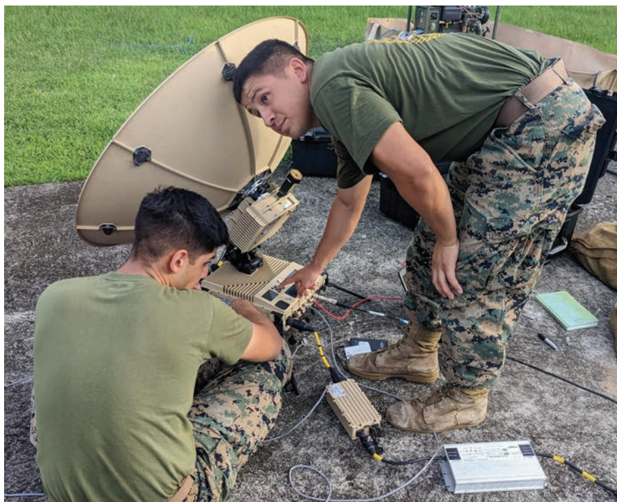
MCWS-X Day. Marines with 3d MarDiv Communications Company establish a Marine Corps Wideband Satellite Expeditionary terminal as part of an expeditionary communications node. (Photo provided by author.)
