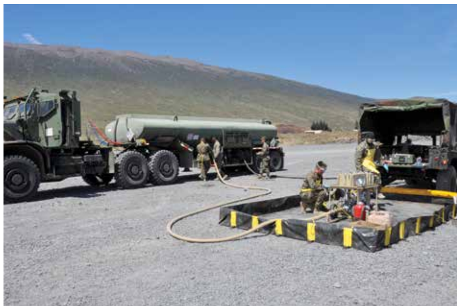
Marines and Soldiers additize fuel in a tank truck at Pohakuloa Training Area, HI, using the Marine Corps expeditionary mobile fuel additization capability prototype system during the RIM of the PACIFIC Exercise, 18 July 2018. (Photo by author.)
