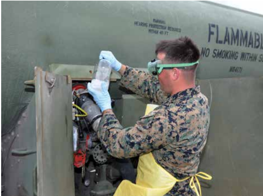
Sgt Grable examines a sample of fuel before conducting laboratory testing to ensure it meets military specifications during the RIM of the PACIFIC Exercise, July 2018. (Photo by author.)
