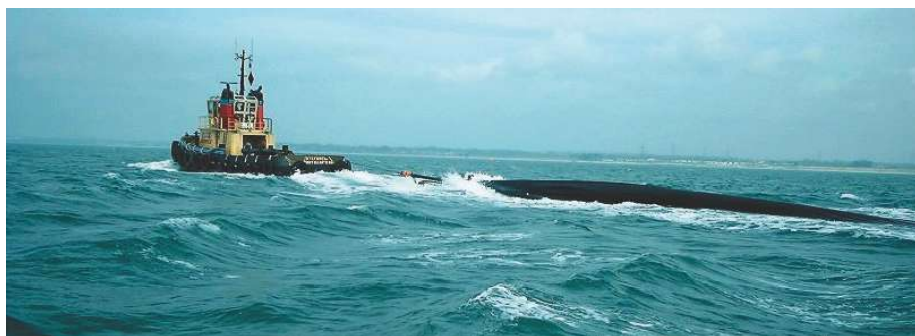
Figure 5. Dracone Barge. (Figure provided by author.)
