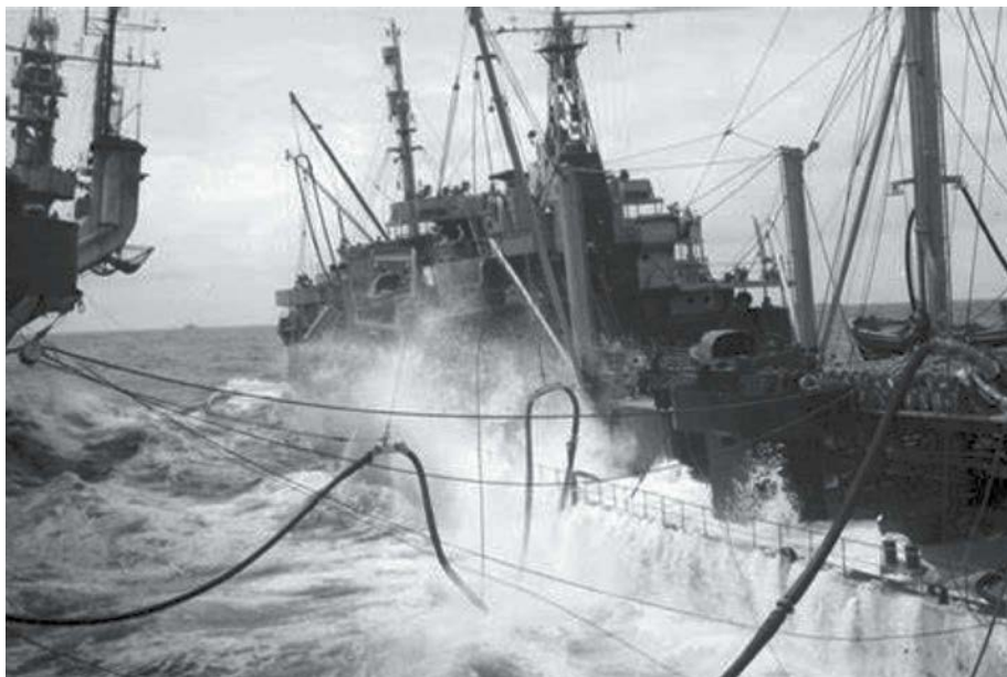
USS Kawishiwi (AO-140) fleet order conducting underway fuel replenishment. (Photo from navymemorieships.com .)
