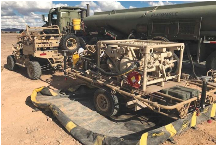
The Marine Corps tactical air ground refueling system. (Marine Corps photo.)
