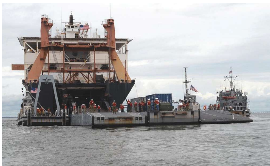
NAVELSG Sailors man a Roll On/Roll Off Discharge Facility (RDDF) while conducting lighterage operations during in-stream offload of vehicles and equipment. (Photo by Chief Petty Officer William Parker.)
