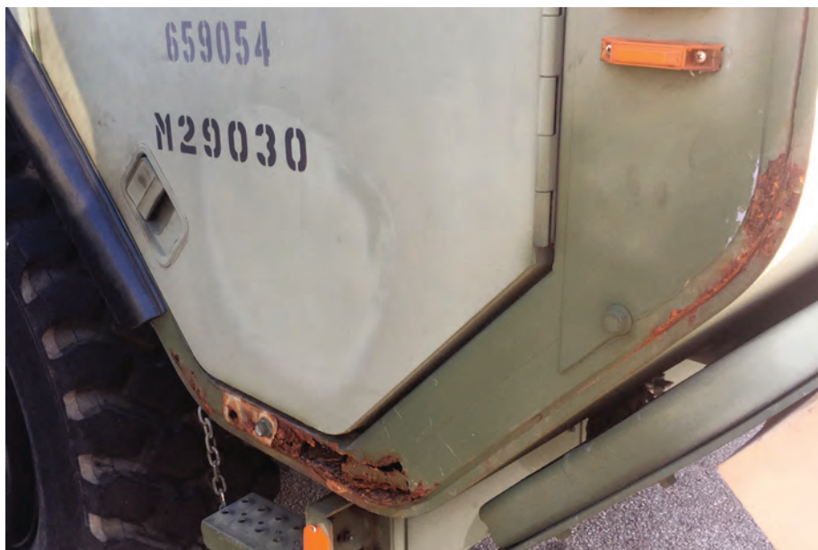
Rust and corrosion exacerbates readiness issues. (Photo by author.)
