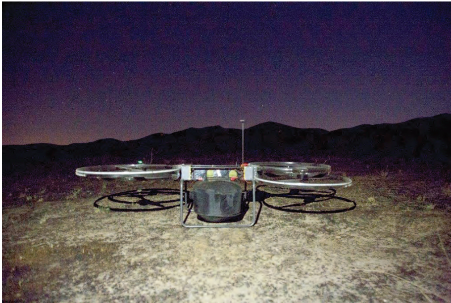
The joint tactical aerial resupply vehicle is being tested by 1stMRB as a potential technical solution for rapid resupply. (Photo by Sgt Salvador Moreno.)
