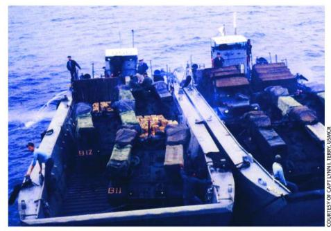
Two LCUs, above, loaded with platoon vehicles and an LVPT, right, floated off the ship from its well deck upon arrival at White Beach, Okinawa.
