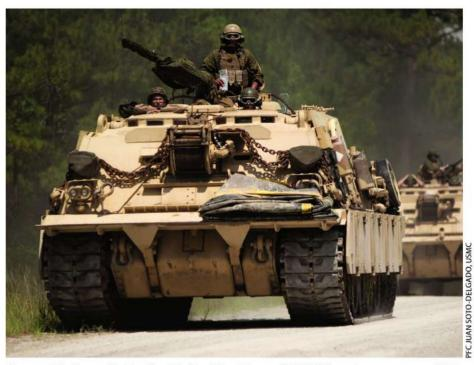
Reserve Marines with Fox Co, 4th Tank Bn drive an M88A2 Hercules recovery vehicle to a landing zone during a field exercise with elements of 2d Tank Bn at MCB Camp Lejeune, N.C. The M88A2 has the ability to tow tanks that weigh up to 70 tons.
