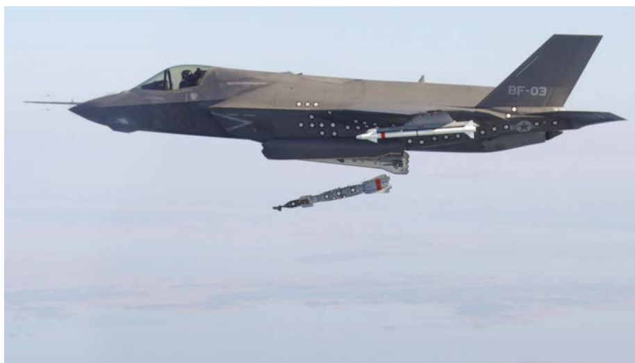
F-35B test aircraft BF-3 completed the first aerial weapons release of an inert 500-pound Guided Bomb Unit-12 over a test range in 2012. This was the first GBU-12 Paveway II Laser Guided Bomb release for any variant of the Joint Strike Fighter.
