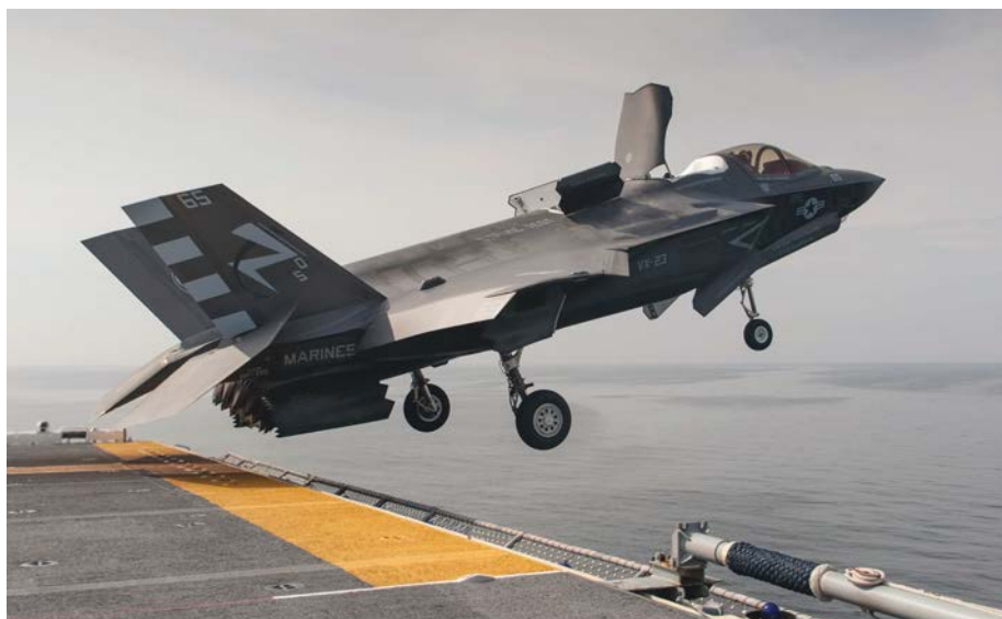
An F-35B test jet takes off from the amphibious assault ship USS Wasp (LHD-1) in August 2013. The takeoff was part of developmental test phase two for the Joint Strike Fighter short takeoff and vertical landing variant.
