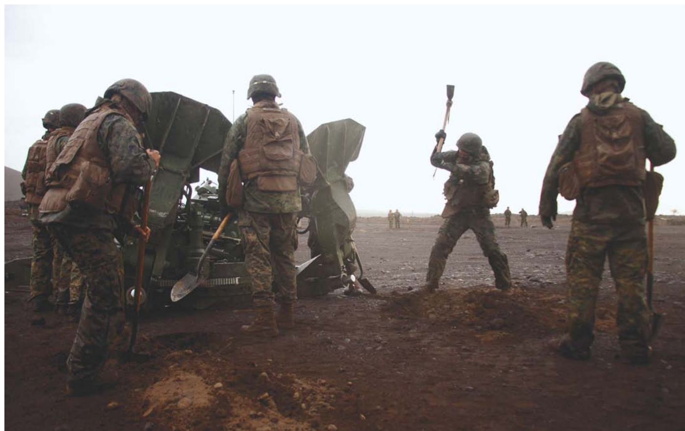
Using shovels and pickaxes, Charlie Btry, 1/12 cannoncocks prepare to emplace the trails of an M777 155 mm howitzer during Operation Spartan Fury. Digging in the spades on the trails helps ensure howitzer accuracy.
