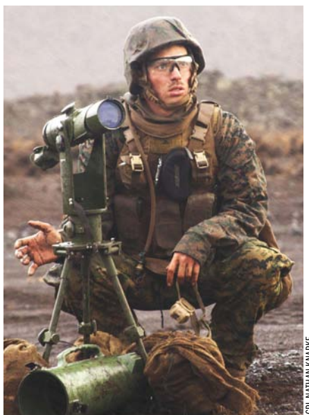
LCpl Zachery Knoebel, a cannoneer with “Charlie” Btry, 1/12, aligns the sights of an M777 155 mm howitzer, using a collimator, or infinity reference point, during Operation Spartan Fury at Pohakuloa Training Area, Hawaii, Feb. 22.
