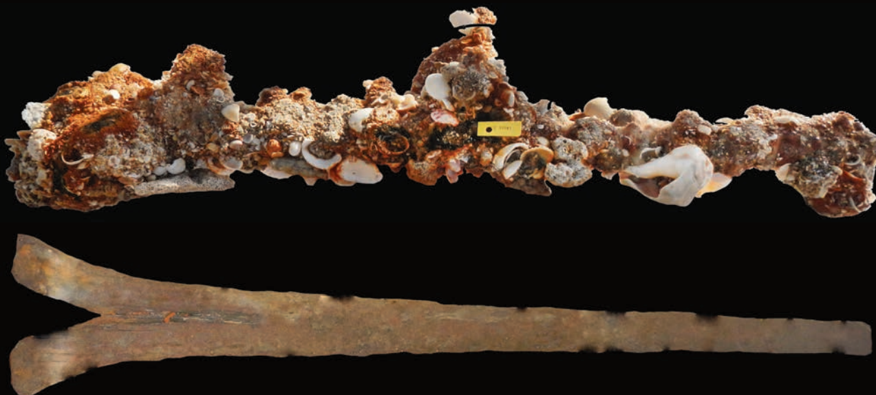
These before-and-after photos show the restoration of a ship's crowbar, which was found on July 6, 2012. Conservators work diligently to restore the items that are recovered from the 1715 fleet.
