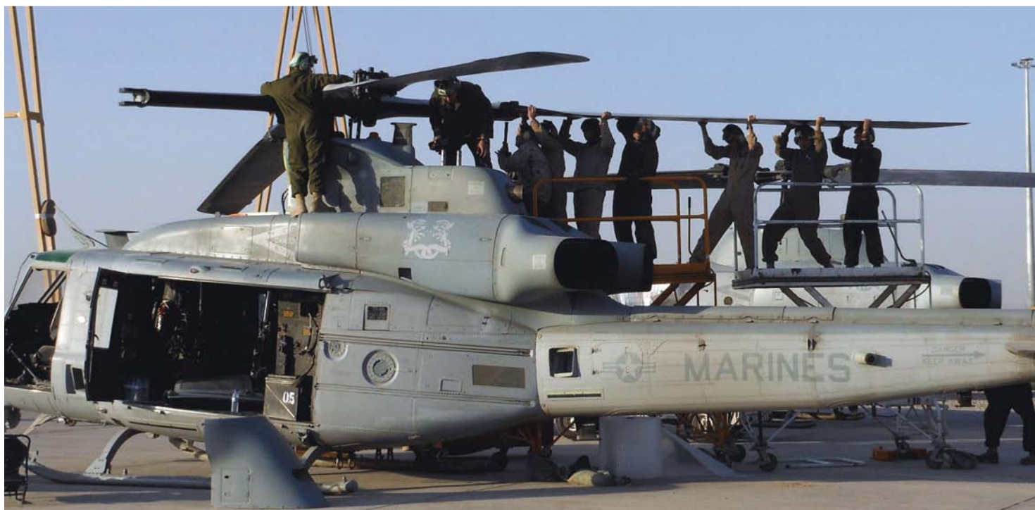
Small-unit leadership, small-unit team work and pretty good-sized muscles are what it takes to fit a main rotor blade into a UH-1Y Super Huey rotor head during repairs at Camp Bastion. Leathernecks of HMLA-369 have it all, including quality assurance, in the environs of Afghanistan. (Photo by GySgt Aaron Jameson)
