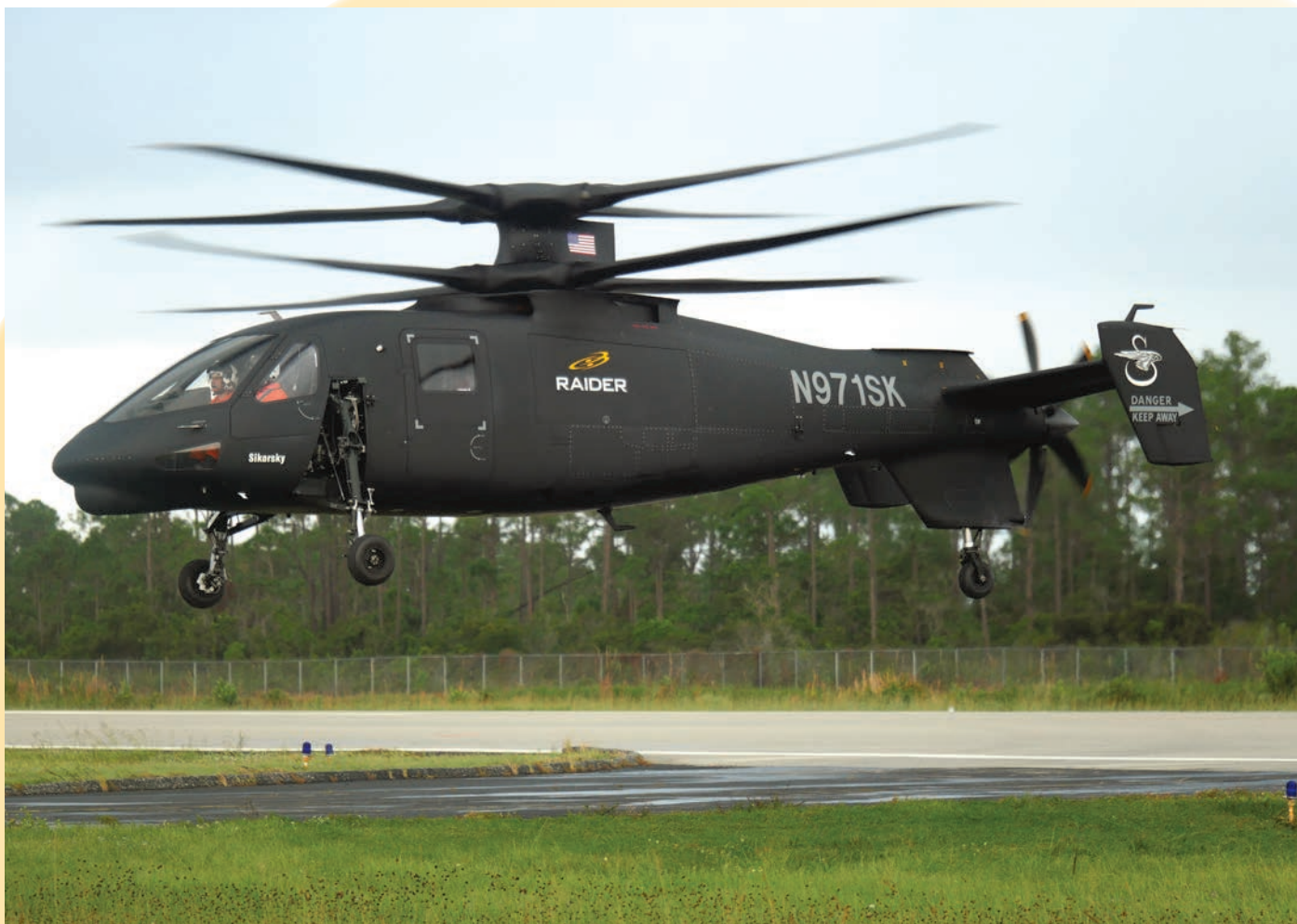
The S-97 RAIDER is one of Sikorsky's newest projects. The helicopter has a coaxial rotor design and is capable of being developed into a unique multimission configuration. It is expected to reach cruise speeds of up to 240 knots (276 mph).
