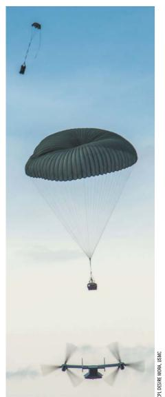
autonomous guidance unit, a parachute, and electric motors to land cargo precisely on its target points by setting coordinates into the system. It has been in testing since the early 2000s and will allow loads to be dropped from higher altitudes, ensuring increased safety for both pilots and ground troops in combat environments.
