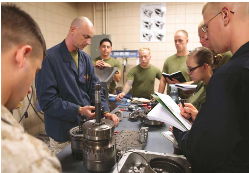
GySgt Zachary Reilly, an instructor in the Motor Transport and Maintenance Instructional Company, Logistics Operations School, MCCSSS, explains to students the disassembly of a valve body on a transmission during a practical-application exercise. (Photo by Sgt Mark E. Morrow Jr.)
