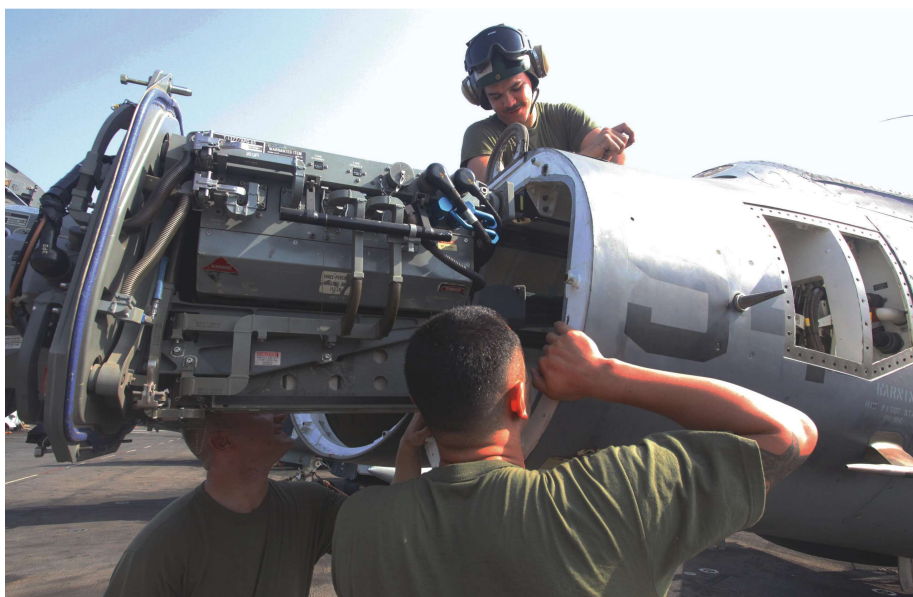
Above: The AV-8B Harriers of VMM-261 (Rein) also receive routine daily maintenance, as these fixed-wing aircraft airframe mechanics inspect, maintain and repair aircraft hydraulic/pneumatic and structure systems while embarked on USS Iwo Jima .
