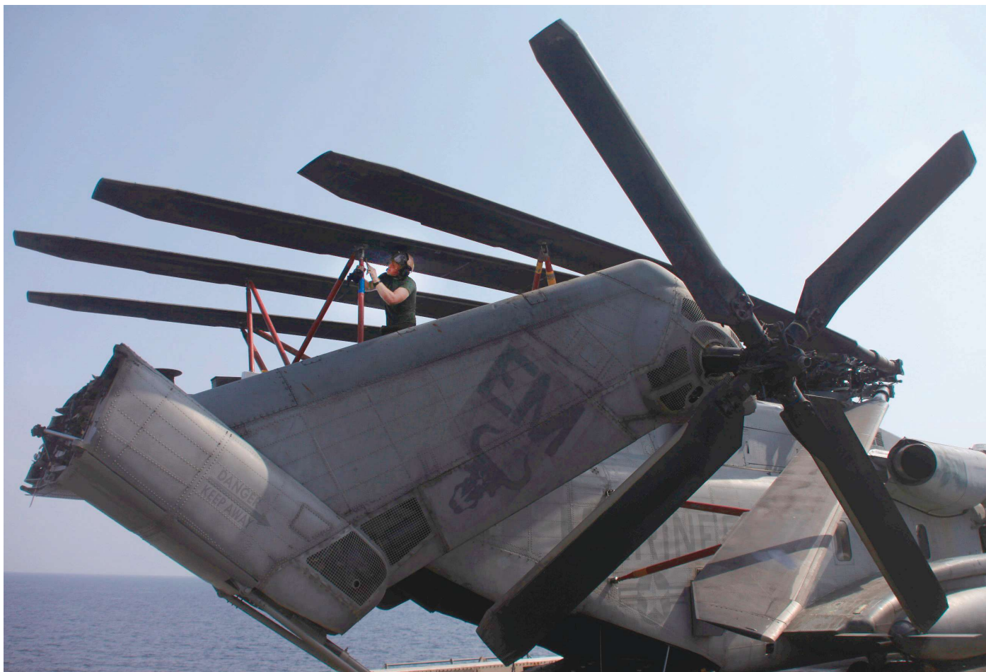
Cpl Lonnie Bowen, a flight-line mechanic with VMM-261 (Rein), 24th MEU, performs corrosion prevention maintenance on a CH-53E Super Stallion aboard USS New York (LPD-21) while under way in September 2012.
