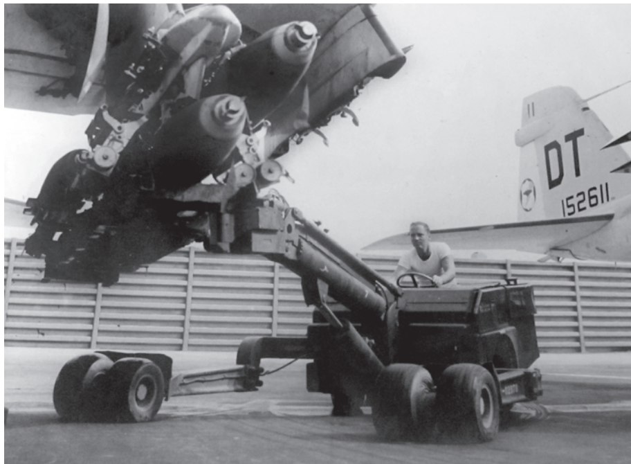
SSgt Lewis R. Souder operates a hydraulic bomb loader while moving a rack of 500-pound bombs under an A-6A Intruder.
