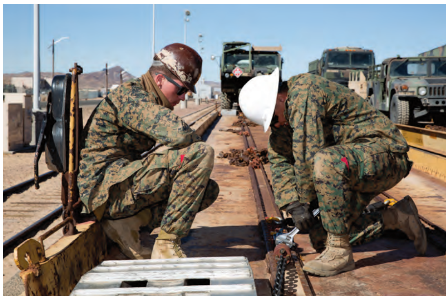
Marines training at the Rail Operations School tighten railcar hardware prior to loading Army vehicles, Feb. 4, 2016.
