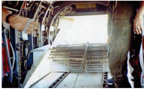
The swinging ladder was made of aluminum rungs and wire and was designed to roll up on the floor of a helicopter and kick off the tail when needed, unraveling to the ground. (Photo courtesy of Dave Thompson)
