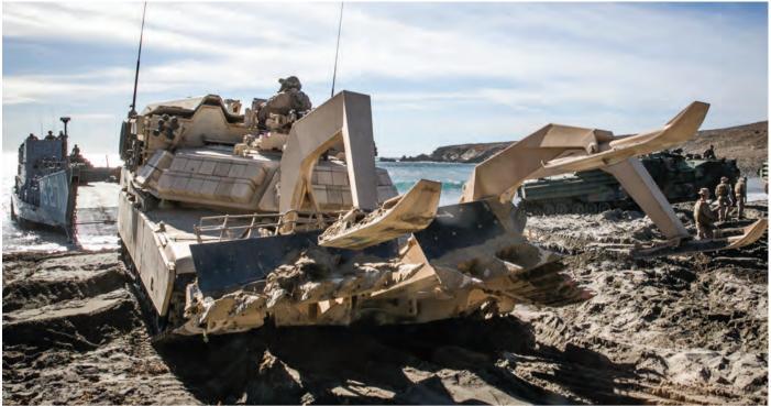
Marines with 1st Combat Engineer Bn, 1stMarDiv, conduct the first amphibious landing in an ABV with the Modified Full Width Mine Plow prototype during Exercise Steel Knight at MCB Camp Pendleton, Calif., in December 2017.
