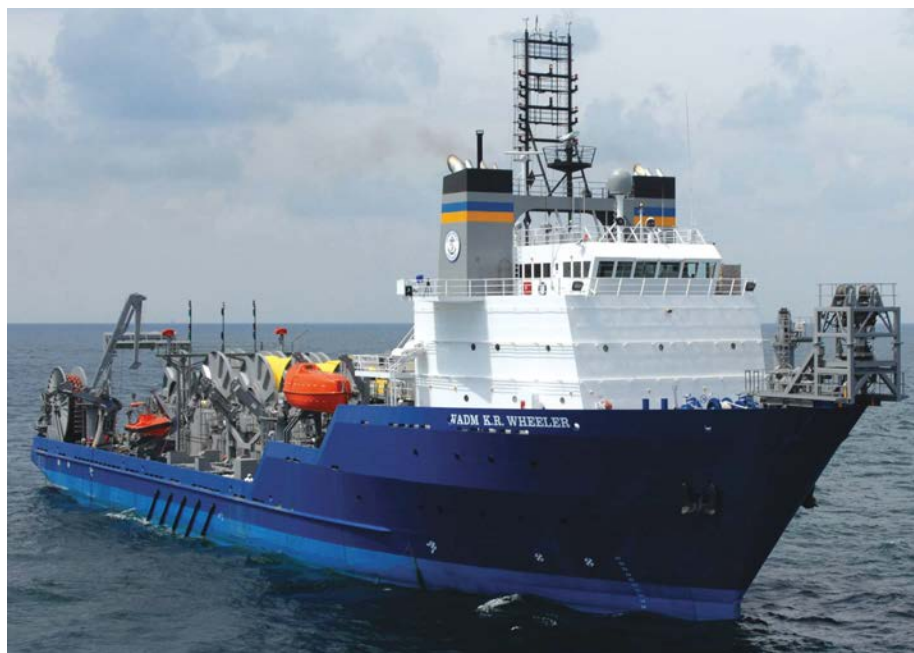
The USNS VADM K.R. Wheeler is an offshore petroleum distribution ship that can pump fuel to facilities from up to eight miles offshore. (Photo by Military Sealift Command.)
