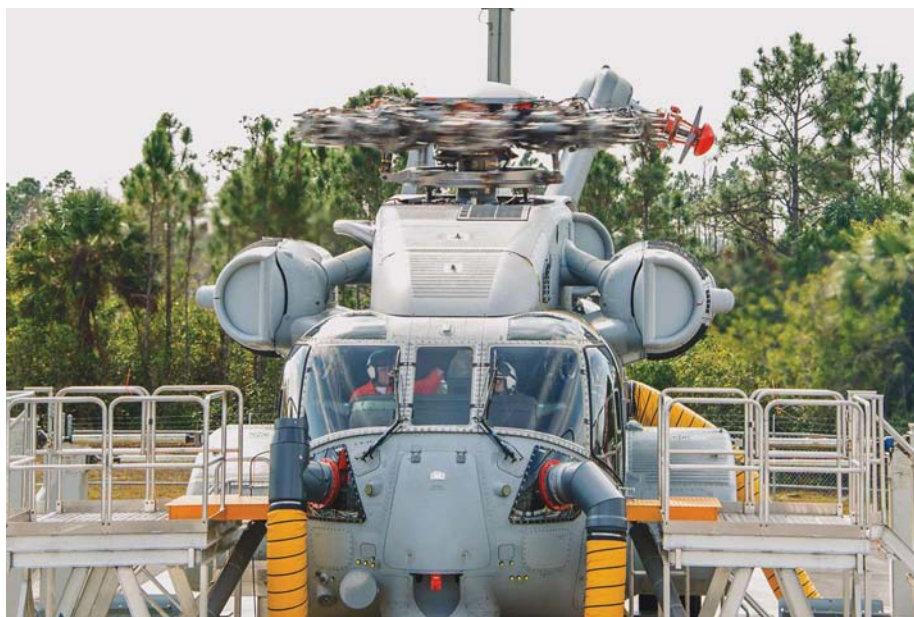
Integrated Test Team pilots, Steve McCulley of Sikorsky Aircraft Corporation and LtCol Jonathan Morel of HX-21, spin the rotor head of the CH-53K Ground Test Vehicle for the first time. (Photo provided by Department of Aviation, HQMC.)
