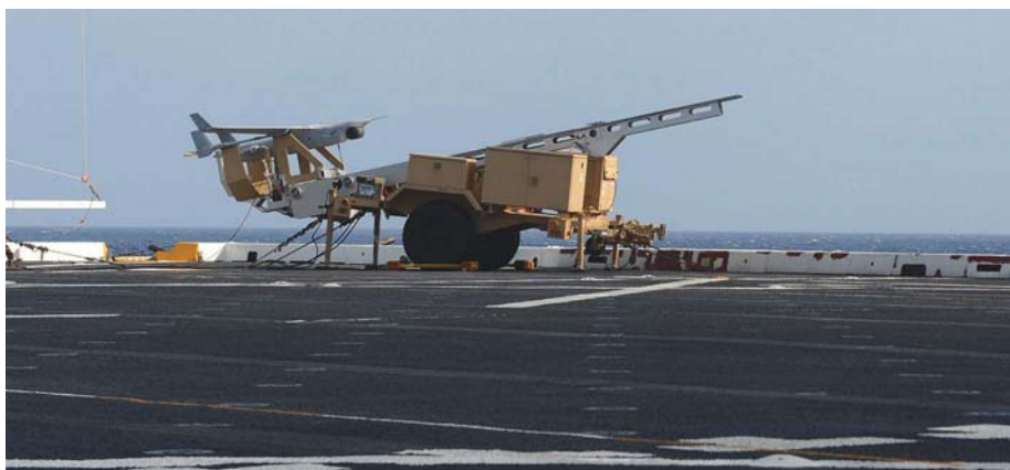
A Blackjack readies for launch aboard amphibious shipping. Its 35-pound payload bay can host an EW capability. (Photo provided by Insitu, Inc.)
