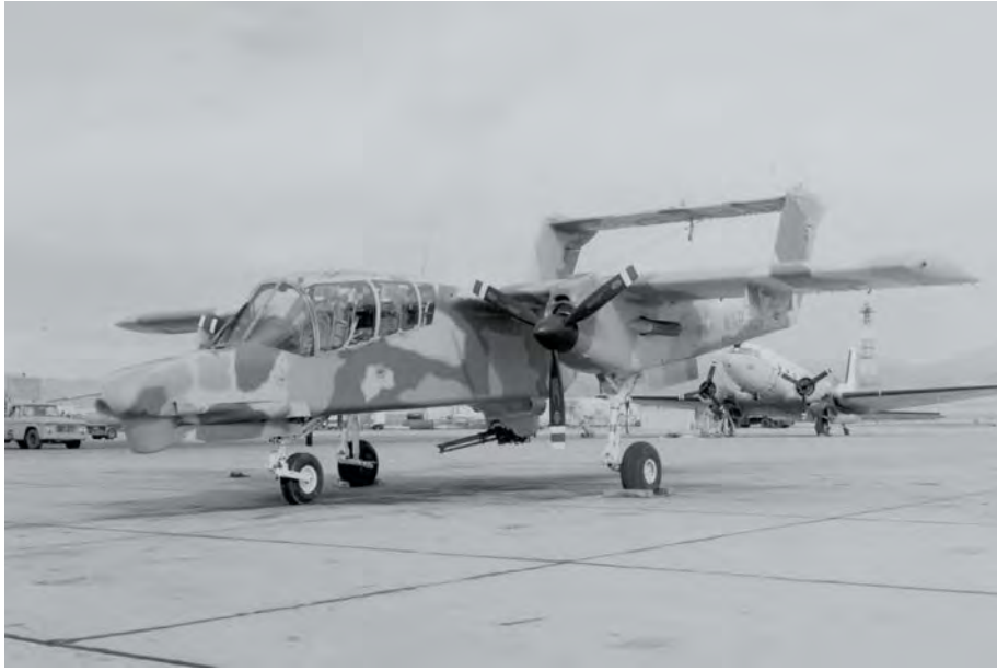
The YO-10D's nose was extended 30 inches to accommodate the FLIR turret and its armament sponson was replaced by the flexible 20mm cannon to form the NOGS configuration. (Photo by Hughes Aircraft Company, January 1971.)
