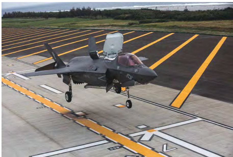
A F-35B Lightning II from VMFA-121 performs a vertical landing during field carrier landing practice at le Shima Island, Okinawa, Japan. (Photo by LCpl Alexia Lythos.)
