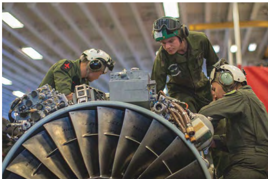
Marine F402 engine mechanics with VMM-163 (Recon), 11th MEU, prepare an engine for installation on an AV-8B Harrier aboard the USS Boxer (LHD-4). (Photo by LCpl Dalton S. Swanbeck.)
