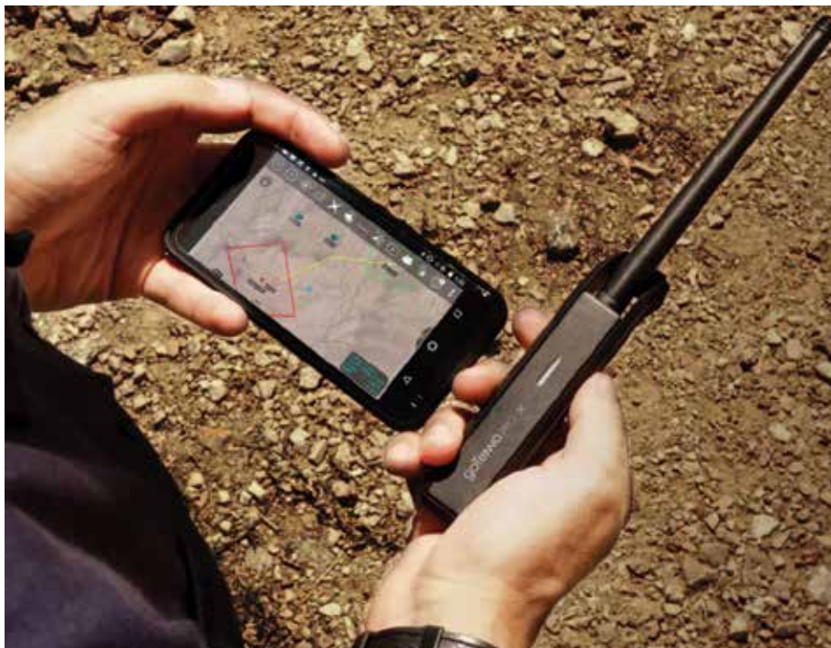
Above is a picture of an individual employing ATAK in a rural environment via goTenna's ATAK plugin and mesh network (goTenna, Inc., 2021). (Photo provided by author.)
