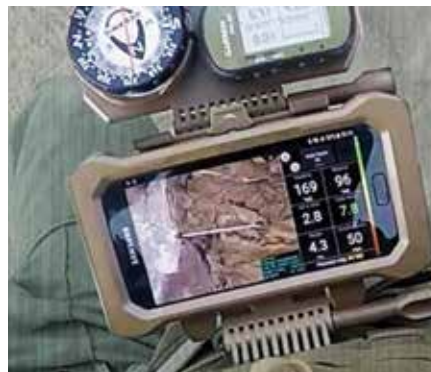
Above is an image of an Android Phone with the Android Tactical Awareness Kit (ATAK) software depicted on the screen being worn on an operator’s plate carrier for quick access. (Photo provided by author.)
