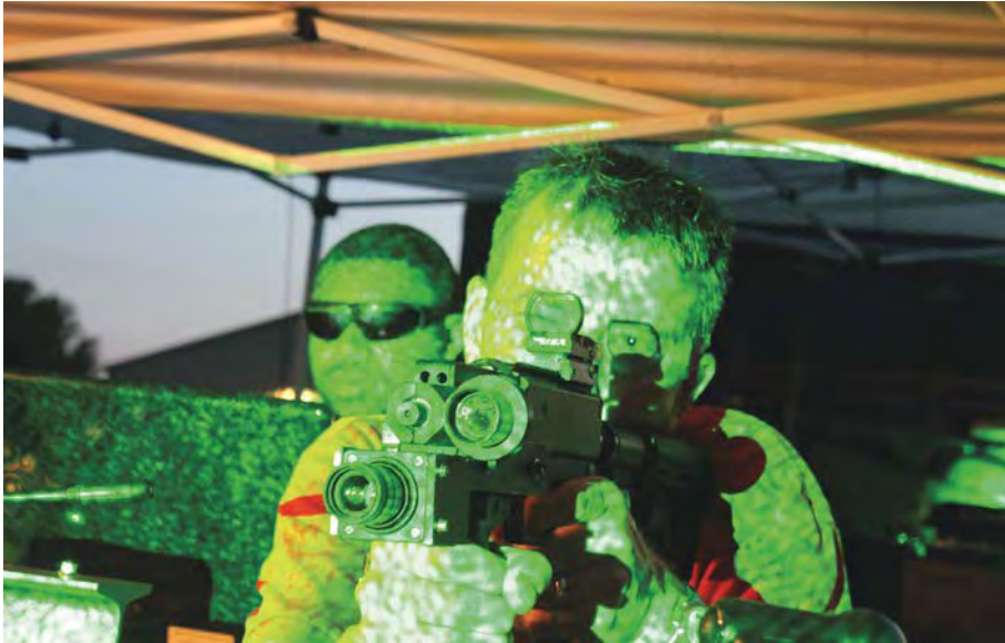
The ocular interruption system is a light emitting, non-damaging, eye-safe device fielded to warn and suppress individuals at a 10-500 meter standoff. (Left photo courtesy JNLWD; right photo by Mimi Ho, JNLWD.)
