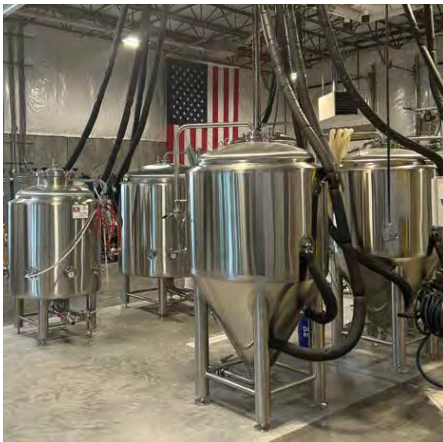
Full Distance Brewing’s five-barrel brewhouse can brew up to 155 gallons of beer at a time.
