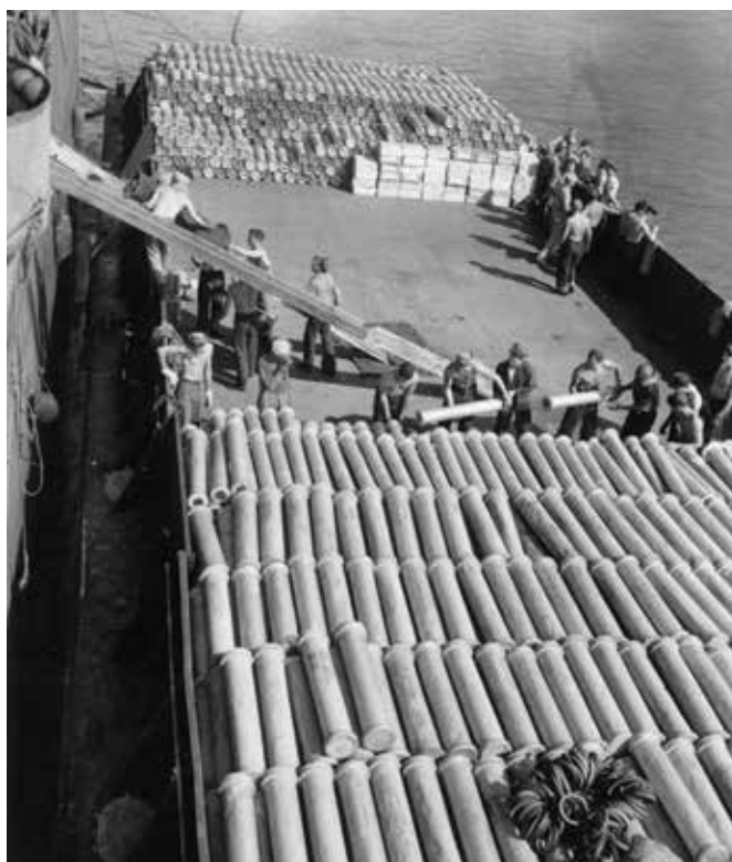
Back at Tulagi anchorage in early July, Honolulu 's ammunition handlers are reloading thousands of main battery 6-inch ammunition. The 6-inch gun fired semi-fixed ammunition, consisting of a projectile and a separate brass propellant cartridge.
